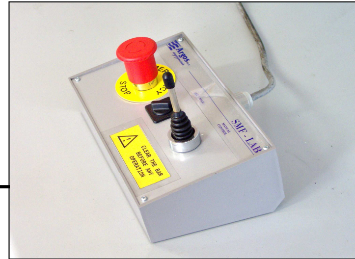
Emergency and control console
