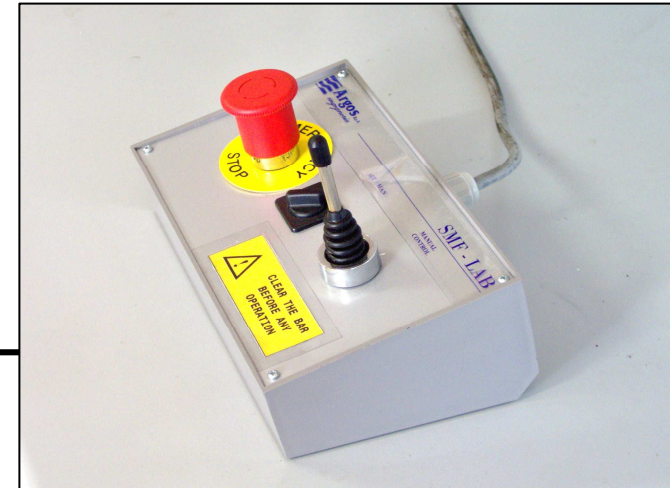
Emergency and control console
