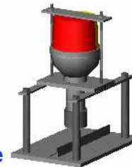
Elevated lights support
