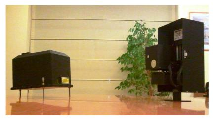
In order to re-calibrate the SMF/PAPI, a 2 step automatic elevation test is required, measuring the laser beam at 3° and 6° approximately (proper values are displayed by the system software). The provided calibration software executes the tests automatically and calculates new calibration parameters for the SMF/PAPI instrument.
