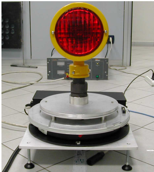
Fig.6 - Elevated light Stand – Approach Light
